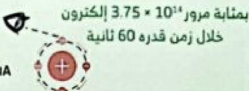
$$I = \frac{Q}{t} = \frac{N \cdot e}{t} = \frac{3.75 \times 10^{14} \times 1.6 \times 10^{-19}}{60} = 1 \times 10^{-6} \text{ A} = 1 \mu\text{A}$$
